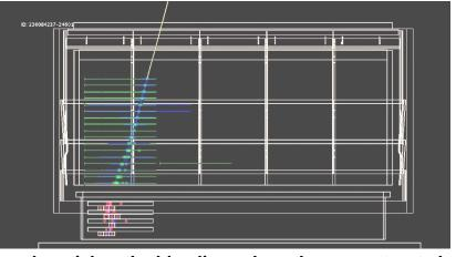
The green crosses show the detected positions of the charged particles, the blue lines show the reconstructed track trajectories, and the yellow line shows the candidate gamma-ray estimated direction. The red crosses show the detected energy depositions in the calorimeter.
