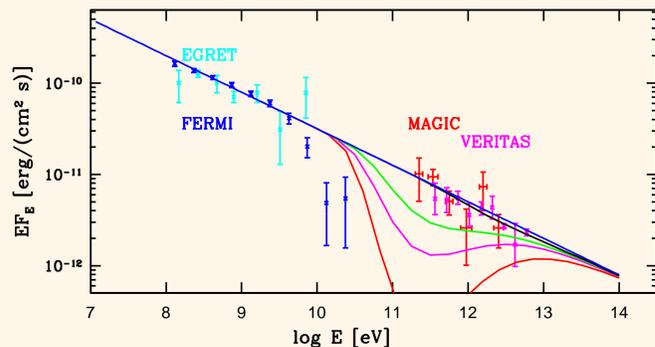
Figure 1: Attenuation of LSI +61° 303 spectrum due to the  $\gamma\gamma$  pair production at different orbital phases. Blue line is an extrapolation of a GeV spectrum before the cut-off. Black, and red lines shows the effect of  $\gamma$ -ray absorption at superior and inferior conjunctions, while green and magenta lines correspond to intermediate ( $\varphi = 0.6$  and  $0.8$ ) phases.
