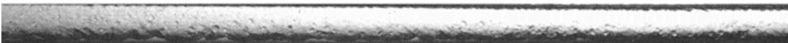
Fig. 5. Flow pattern of CO 2 ( D_p = 2.0 mm, p = 5.0, 6.5 MPa, flow direction: left to right).
