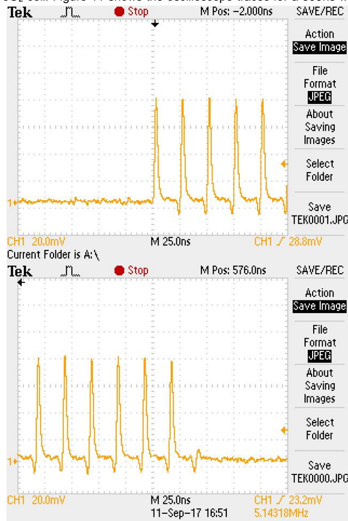
Figure 11. Top: Rising edge of the burst; Bottom: Falling edge of the burst.
