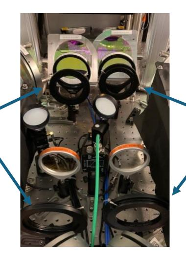
Final East beam path for legs GH (adjustable) and IJ (fixed) through alignment iris's
