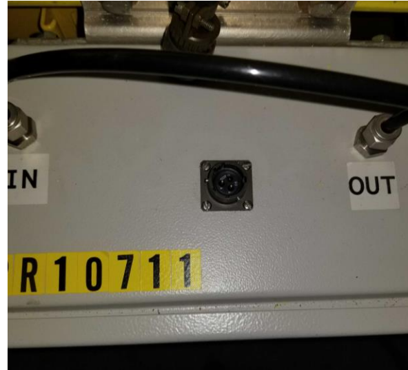
Figure 1 : Profile Monitor Terminal Block with connections Figure 2 : Profile Monitor Airbox Connector
