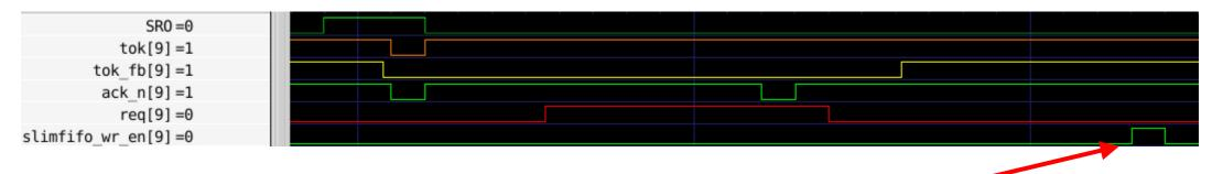
The ADC conversion process induces a latency  $\rightarrow$  wrEn for the data word (ADC word + addr is issued 'late')
