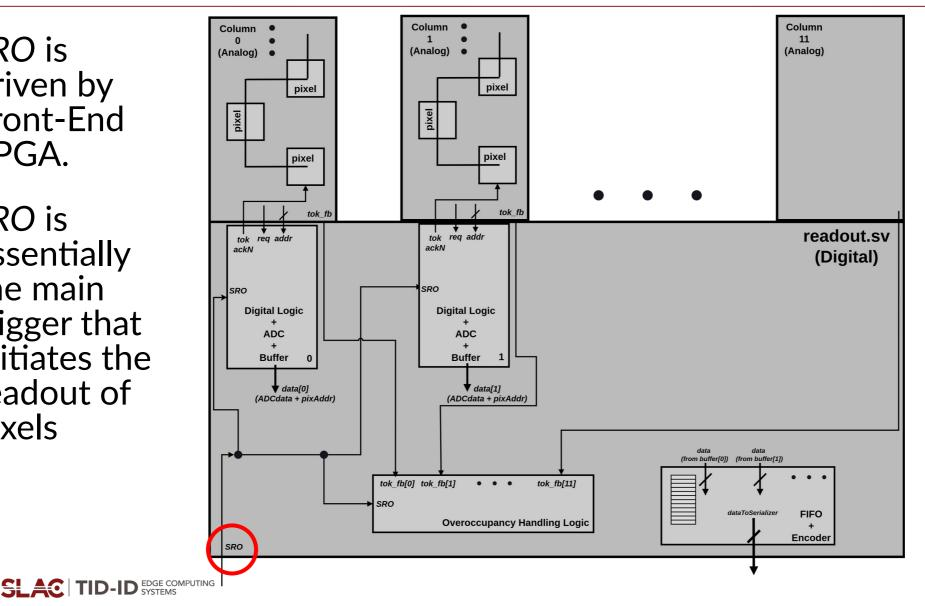
Each pixel column accepts the SRO in the form of a token (tko). If a pixel has data, it requests to be digitized (req). Data are then converted and buffered
