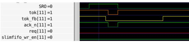
Overoccupancy  $\text{Error} \rightarrow \text{receive new } SRO \text{ before } tok_fb \text{ goes high} OR \\ \text{receive new } SRO \text{ before last } FIFOwrEn \text{ is issued}$
