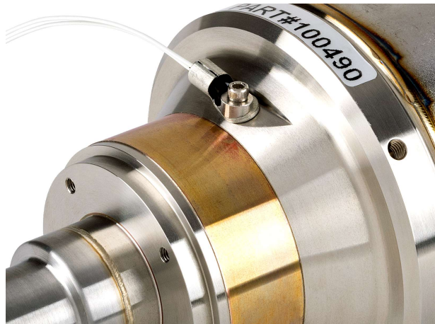
Figure 10. Thermistor Screwed onto the Cryocooler with 3-48 screw
