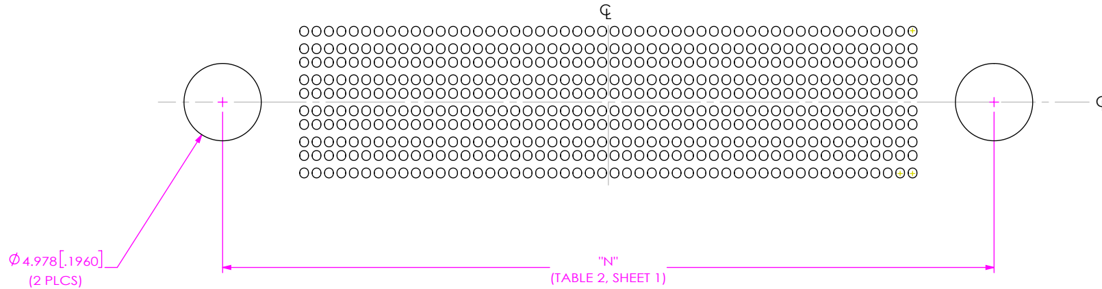
FIG 8 (GUIDE POST OPTION) SEAM8-50-SXX.X-XXX-10-1-GP-X-XX & SEAM8-50-SXX.X-XXX-10-3-GP-X-XX STENCILS SHOWN (SAME AS FIG 10, EXCEPT AS SHOWN) ALL DIMENSIONS ARE SYMMETRIC ABOUT THE CENTERLINE.
