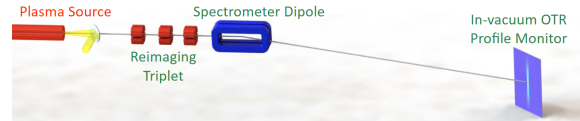
FIG. 1. Higher energies are more “rigid” meaning they are bent less by the dipole while lower energies are bent more - this gives a profile the transverse size of the beam as a function of the beam energy.
