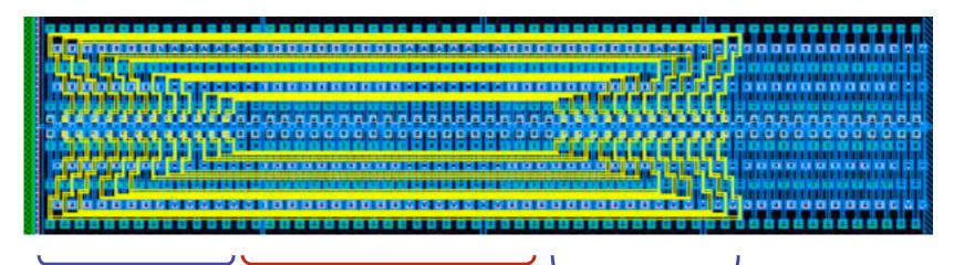
Bumps connecting offset pixels and ASIC cells: chip covers only a fraction of the sensor area.
