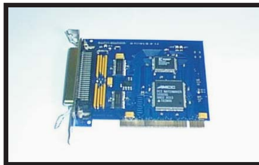
Figure 7: Picture of the BB-PCI interface card. A free standard PCI slot is needed for the installation. Supported OS are windows 95 / 98 and windows NT 4.0. Drivers for windows 2000 are not yet available.
