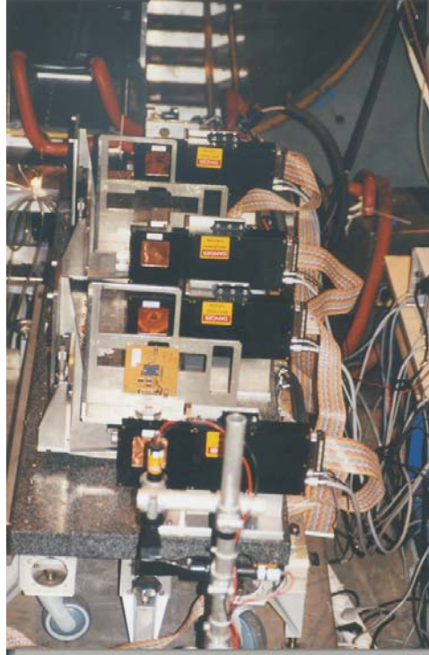
Figure 68: The BAT inside the H8 testbeam area at CERN. The four modules are fixed to a solid support each mounted on a stone table. The H8 testbeam magnet can be recognized in the background. A DUT (ATLAS FE single chip) not yet fully wired is located between the first and the second BAT nodule. The trigger scintillators are also visible.
