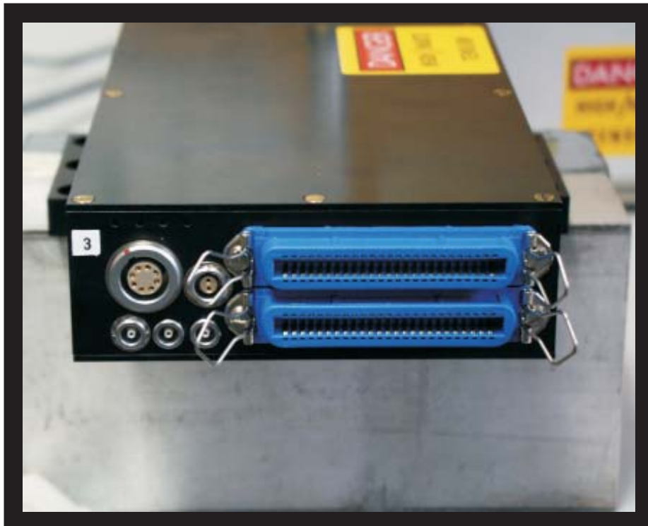
Figure 14: Photography of a module's back side holding the connectors. The LED are hardly visible, because they are not lit. The blue IEEE 488 connectors have been replaced later by a more reliable type which is black.
