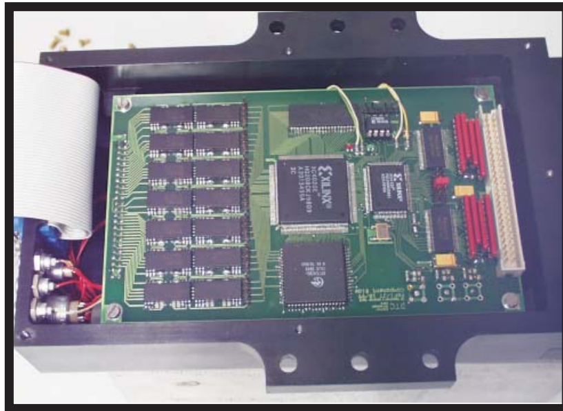
Figure 29: Photo of the DTC card in a module setup. The orientation is the same as in fig. 28. The flat ribbon cable used to connect the PCB with the case BB connectors has been removed.
