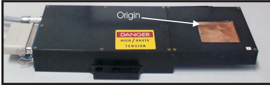
Figure 15: Photography of a fully covered module (front side). The ELEC and DETC covers can clearly be distinguished. The beam window is covered with copper plated capton. The origin of the module coordinates (crossing of strip 1 on N side and strip 1 on P side) is indicated by an arrow.
