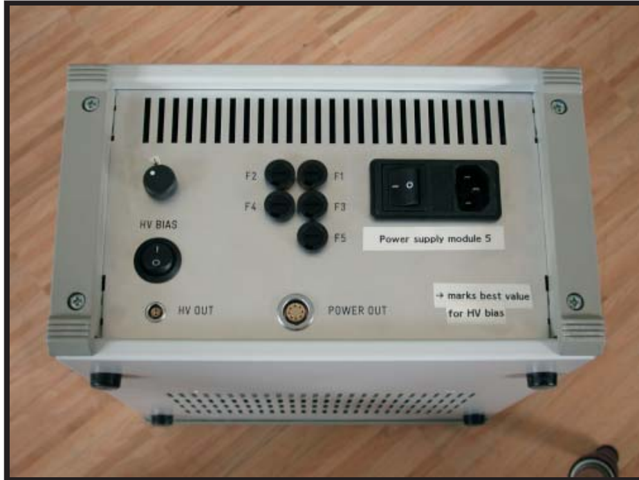
Figure 54: Rear view of a module's power supply. from left to right and from top to bottom: HV bias adjustment potentiometer, HV bias switch, HV bias output connector. Low voltage fuses, low voltage output connector. Line switch, power cord connector and line fuses are sitting together in the rightmost mounting.
