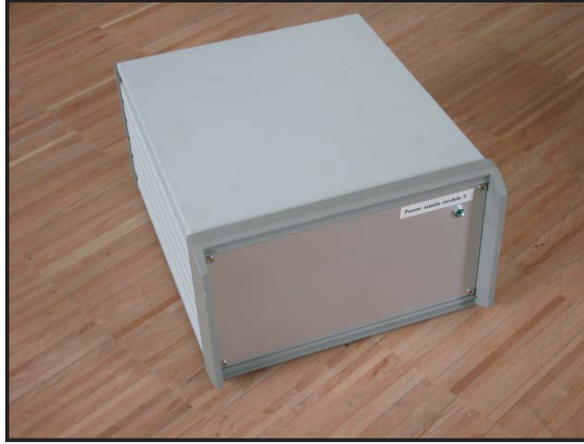
Figure 51: Photo of a module's power supply type NTBONN4. The only item on the front cover plate is the LED indicating system operation. The case size is 25 \times 15 \times 30 \text{ cm}^3 . The cases can easily be stacked.
