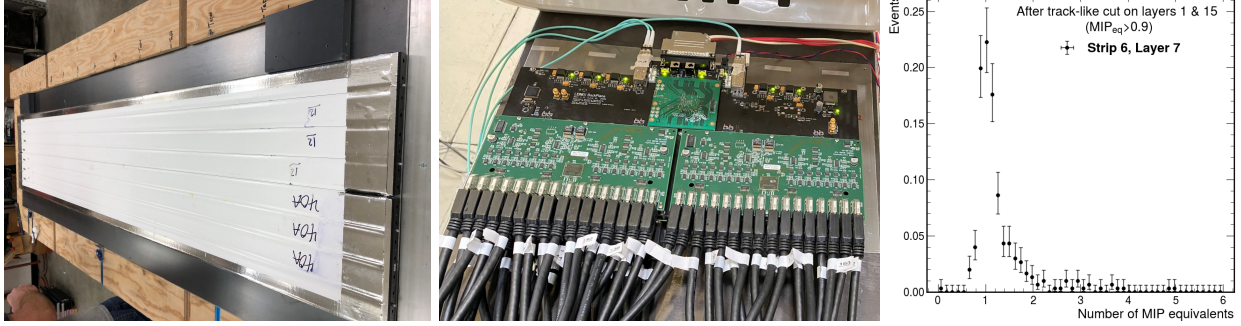
Figure 13: Left: A two quad-bar HCal prototype layer constructed at Caltech with bars fabricated by UVA. Middle: From the test beam set-up: Four HGCRROC boards developed by Lund University mounted (two on each side) on a Backplane board developed by Fermilab, that holds a Mezzanine board developed by University of Minnesota, from which the serialized output is read through optical fibers. Right: The distribution of ADC counts for a single channel (expressed as number of MIP equivalent) from a 4 GeV muon beam run. Muons are required to leave a minimum of 0.9 MIP equivalent in counters in the front and back layers of the HCal.
