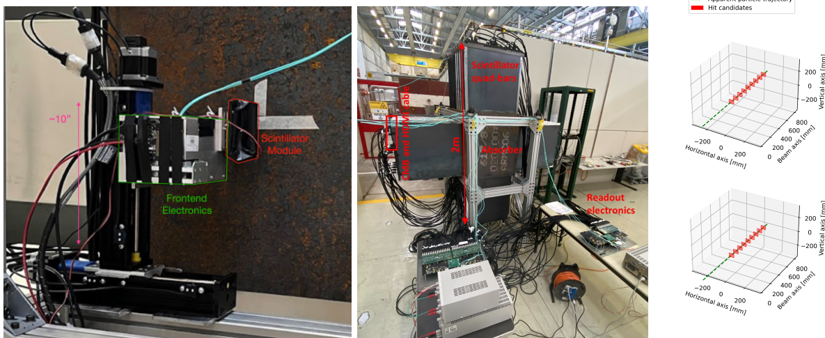
Figure 8: The prototype in the T9 test beam at CERN. Left: The prototype Target Scintillator front end electronics and scintillator module mounted to linear stages. Middle: The back of the HCal prototype with its r/o-electronics on the two tables. Right: Muons crossing the HCal prototype. The red rectangles represent the hits significantly above pedestal. Their location is inferred from the position of a pair of adjacent horizontal and vertical bars. The green line is an estimate of the trajectory of the muons.
