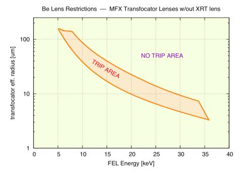
Trip Limits for MFX Transfocator with 333 µm XRT Lens alone
