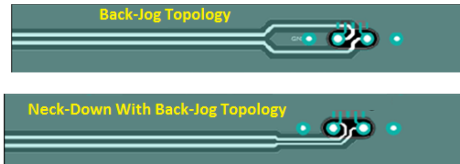
Figure 14. Recommended Single-ended Back-jog and Differential Neck-down with Back-jog Break-out Routing
