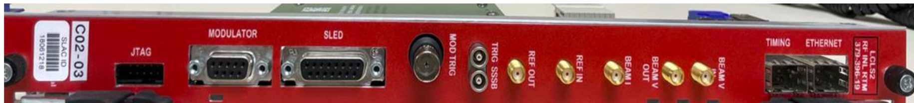
RF Interlock RTM (PC_379_396_19_C02)
