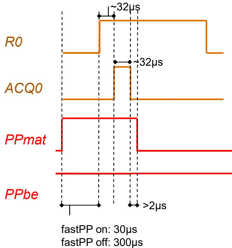
The Back-End by default is always ON. In order to enable the BE Power Pulsing PP\_OCB\_S2D bit (reg10 b0) must be set to 0.
