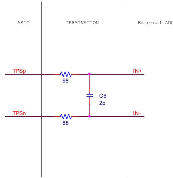
The value of the filter capacitor should be tweaked according to test results.
