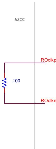
There is a 100 Ohm Termination if SLVDSbit (reg6 bit 4) is 1. (Default is 0 – Open Circuit Termination)
