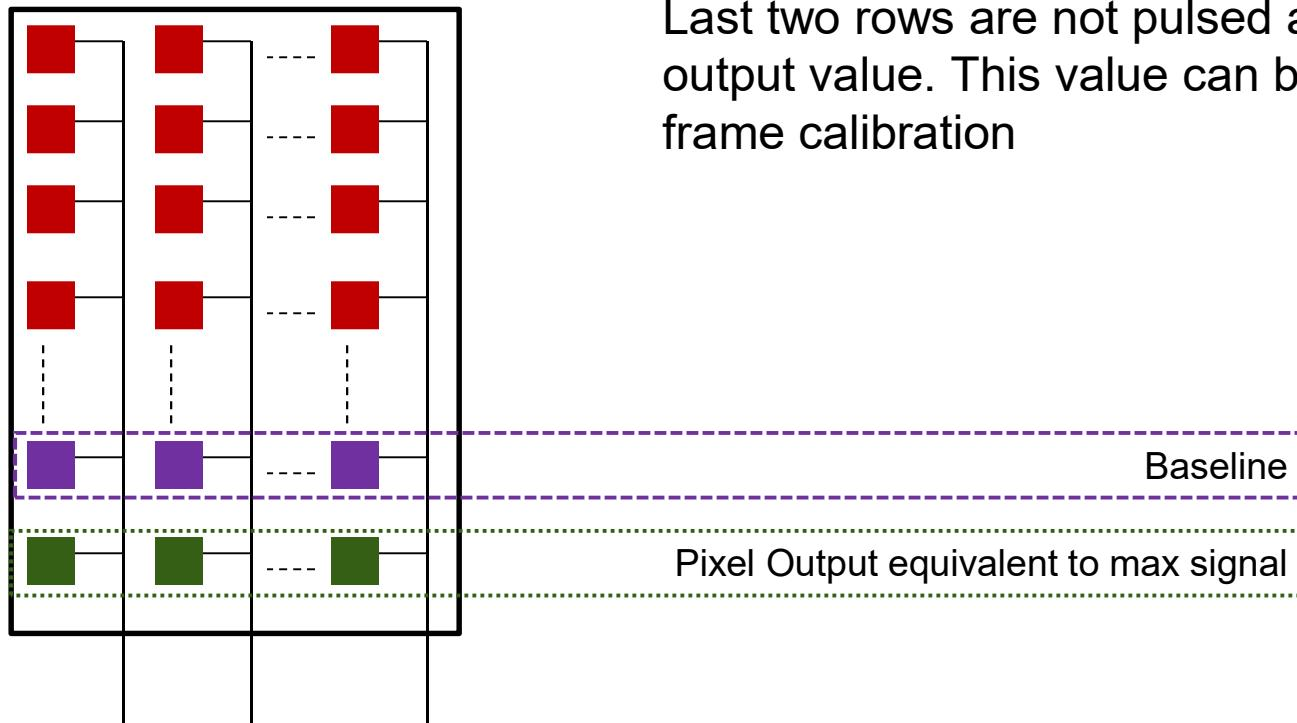
Last two rows are not pulsed and give a fixed output value. This value can be used for an in-frame calibration
