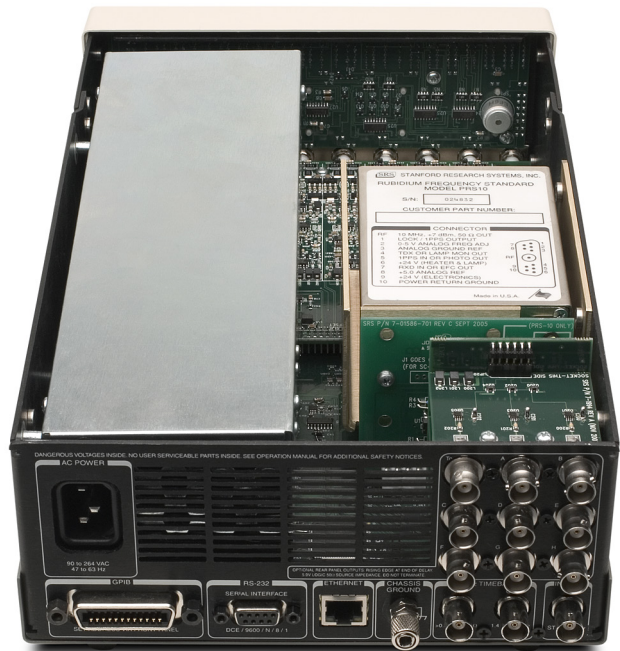
DG645 (cover removed) with optional Rb timebase. Rear panel shows the optional eight-channel outputs.
