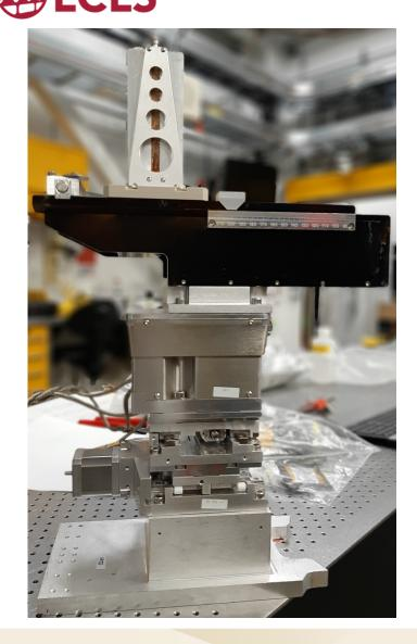
Cylindrically curved graphite crystal spectrometer in von Hamos geometry
