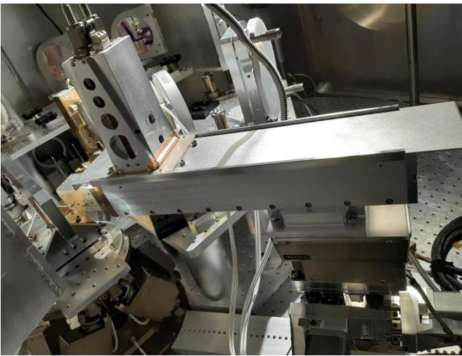
Original version of HAPG spectrometer is available for the X-ray energy range from 4 keV to 8 keV
