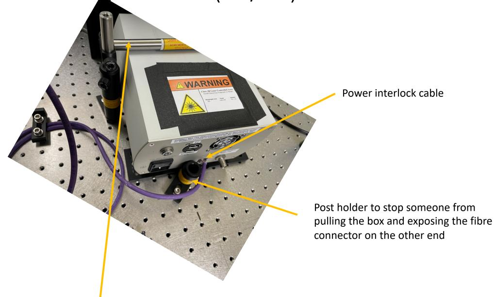
Laser clamped down (post and post holders labelled as laser safety devices)
