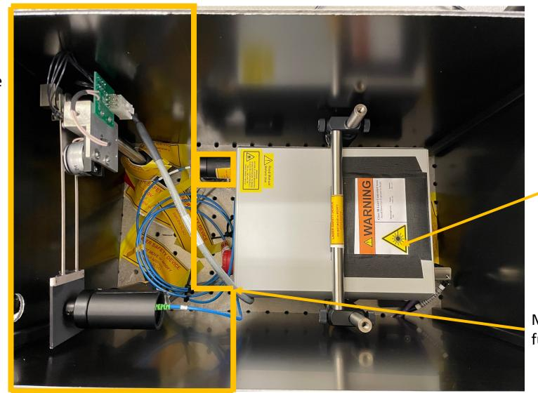
Leave laser controller itself un-enclosed (master key and front button are accessible)
