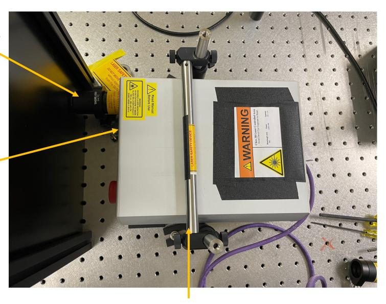
Laser clamped down (post and post holders labelled as laser safety devices)
