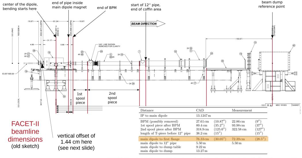
TABLE I. We quote both distances which have been extracted from the CAD drawing (see Fig. 1) and those measured by Lauren/Carsten. Distance from center of magnet to 12" pipe (measured) is given by 28.5" (magnet) + 9" (BPM) + 37" + 127" (two spool pieces) + 15" (T-piece, only CAD value known so far).
