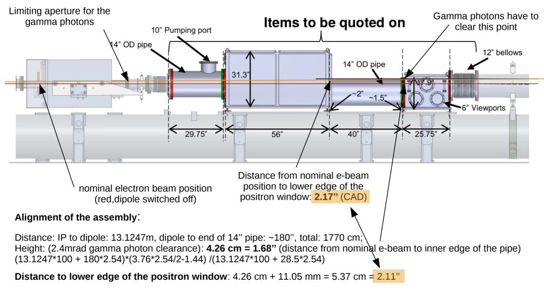
Details left to fine alignment in the tunnel
