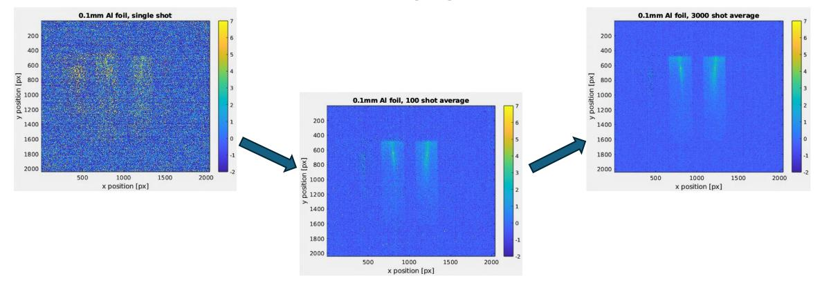
Aluminum foil signal is faintly visible even with a single shot after all other background subtractions
