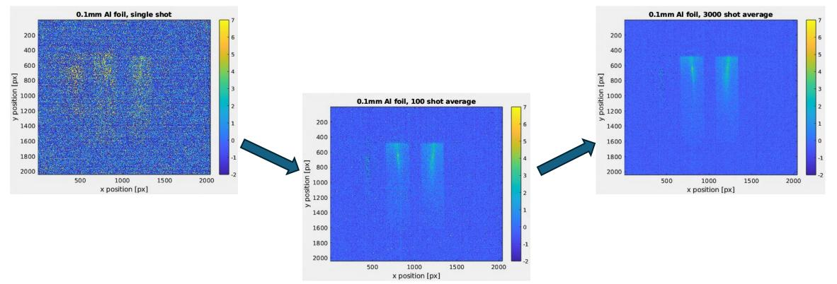
Aluminum foil signal is faintly visible even with a single shot after all other background subtractions
