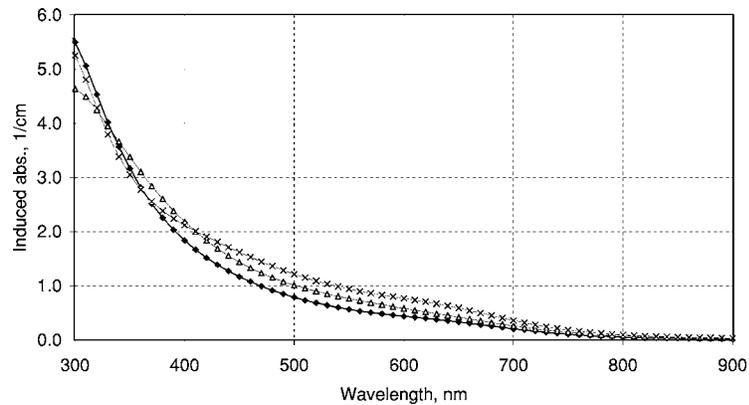
**Fig. 4** Induced absorption spectra of 5-mm-thick samples after 0.6 krad/h dose rate irradiation up to 173 krad:  $\blacklozenge$ , NBK7;  $\blacktriangle$ , BSC; and  $\times$ , S-BSL7.
