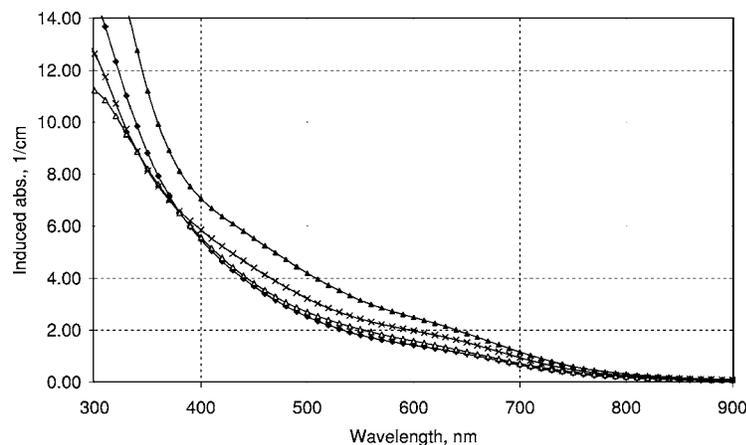
**Fig. 3** Induced absorption spectra of 5-mm-thick samples after high-dose-rate (200 krad/h) irradiation up to 600 krad; curve marking corresponds to  $\blacklozenge$ , NBK7;  $\triangle$ , BSC;  $\times$ , S-BSL7; and  $\blacktriangle$ , K8.
