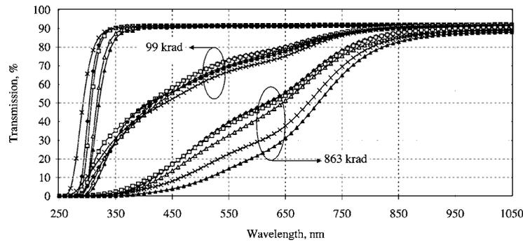
**Fig. 1** Transmission spectra of 5-mm-thick samples; curve marking corresponds to  $\blacklozenge$ , NBK7;  $\square$ , BK7;  $\triangle$ , BSC;  $\times$ , S-BSL7; and  $\blacktriangle$ , K8. The upper set of curves is the initial transmission, the middle and the lower are after exposure to 99 and 863 krad at 2.4 krad/h, respectively.
