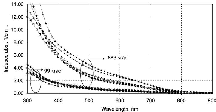
**Fig. 2** Induced absorption spectra of 5-mm-thick samples for 2.4-krad/h dose-rate irradiation:  $\blacklozenge$ , NBK7;  $\square$ , BK7;  $\triangle$ , BSC;  $\times$ , S-BSL7; and  $\blacktriangle$ , K8.
