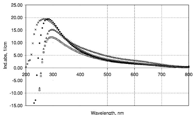
**Fig. 5** Induced absorption spectra of thin samples after low-dose-rate irradiation up to 863 krad as measured 574 days after the end of irradiation:  $\blacklozenge$ , NBK7;  $\square$ , BK7;  $\blacktriangle$ , BSC; and  $\times$ , S-BSL7.
