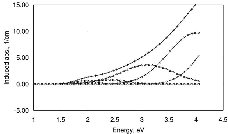
**Fig. 6** Example of the decomposition of an IAS (NBK7,  $D=863$  krad) into individual absorption bands. The maximal difference between the experimental (solid line) data and the synthesized curve (line marked with +) is  $0.05 \text{ cm}^{-1}$  and the average difference is  $0.006 \text{ cm}^{-1}$ . The curves marked with solid diamonds, open squares, open triangles, crosses, and open circles show the contributions of the bands 1 to 5, of which the parameters are given in Table 1.
