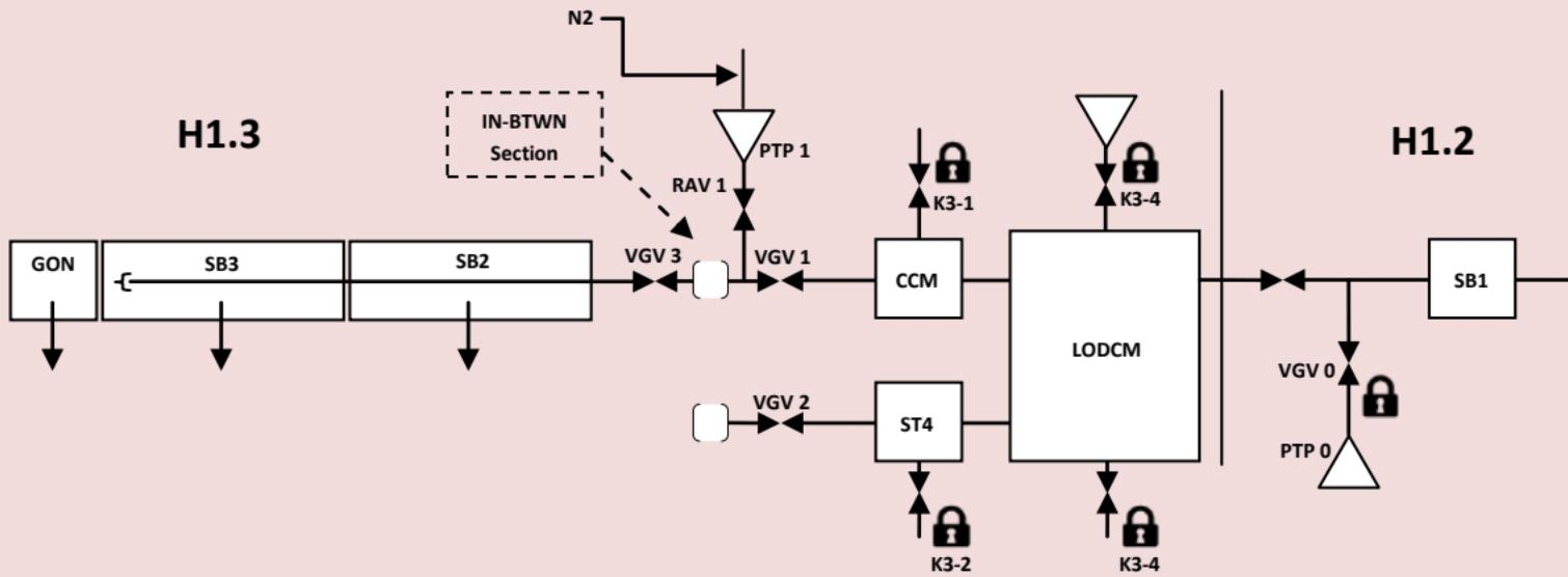
Abbreviations: **VGV** = gate valve, **RAV** = right-angle valve, **PTP** = turbo pump
