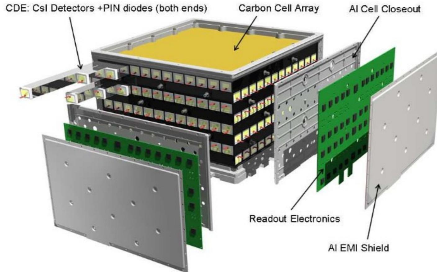
**Each calorimeter tower: 8 layers of 12 CsI bars hodoscopic arrangement read out by photodiodes**
