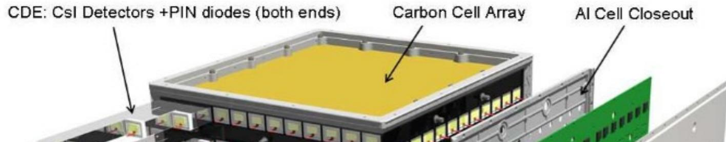
Each calorimeter tower: 8 layers of 12 CsI bars
