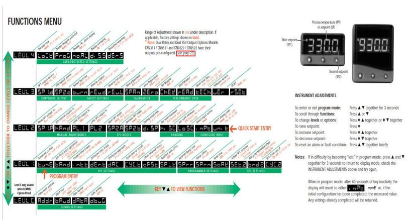
1) Pic.1 shows you how to enter program mode, how to change levels, and how to exit program mode. (also on page 6 of manual)
