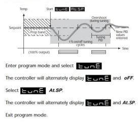
The **TUNE AT SETPOINT** program will now start. The controller will alternately display **Europe** and the process temperature.
