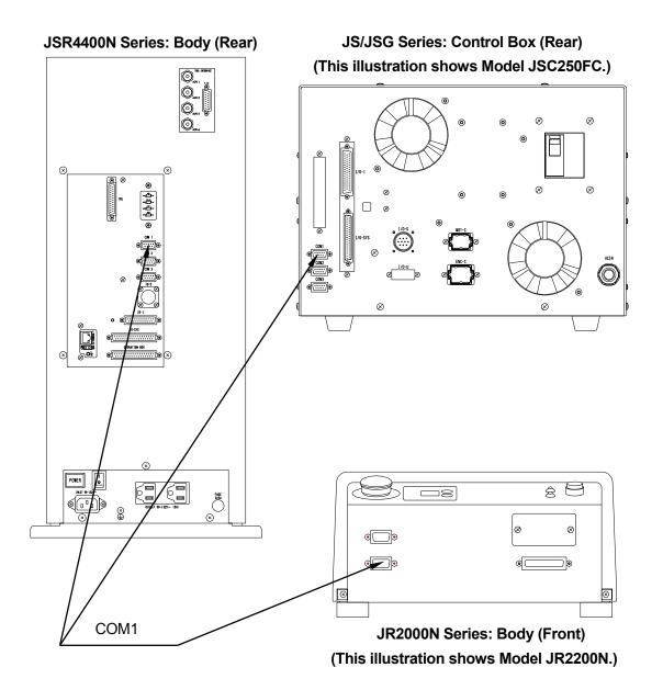
Use a D-Sub 9 pin connector for the robot.
