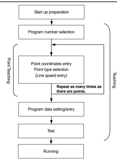
A program is made up of point data which is organized to form a body of program data. Point data consists of the data related to a given location, or "coordinate" as well as the "point type" which describes the method of the Robot's movement to the next point. These form the skeleton of the program, while the point job data (the data consisting of commands to perform operations) which is set to each point adds muscle to the program.
