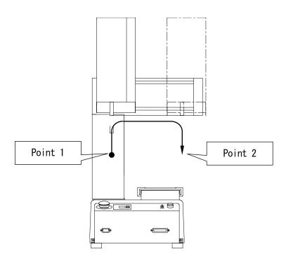
Each point has its respective point type, and the method of movement to the next point varies according to point type. The PTP point type, for example, describes a point which makes a PTP movement to the next point.
