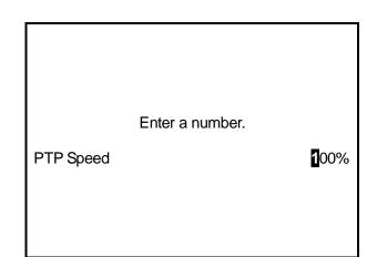
• The recommended PTP speed setting is 20%. You can increase the speed after checking the actual operation.
