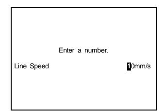
• If you select a point type to go to the next point when using the CP drive, you need to enter the [Line Speed].
