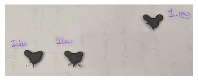
I also recorded a video of this and the results are fairly interesting. Whilst the pressure seems good (based on the size and shape of the starting points of the star pattern), the time the air is on for seems wrong. The glue essentially seems much less runny than when Aidan did this and so needs the air to be on for longer. It might also be that the vacuum is too strong, but I don't want to vary too many pars at once.
