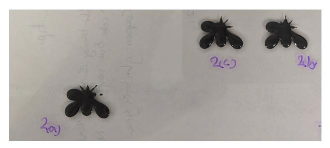
This actually looks much better for the starting points, but the end points are still being cut off... If the pressure is fine, maybe the compressed air is just not blowing the glue for long enough? I'm now going to tru change the air blowing to 2 seconds from one.
