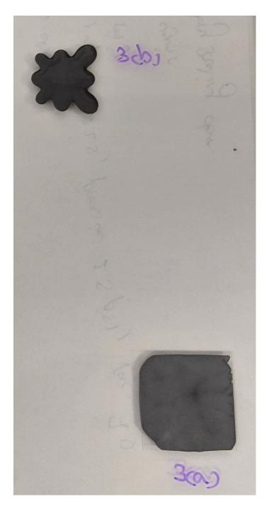
So this is very interesting. The pattern is definitely better but it looks like the ends are still not correct, does the air need to be on for even longer? Matt & I placed a slide on by hand (I placed it, he handled the vacuum) and it's clearly way too much glue. So, what I think I'll do next is increase the time to 2.25 seconds, but drop the pressure a little to get the mass down.
