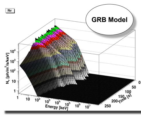
A model produces a 2 dimensional histogram that stores the flux N(e,t) (ph/keV/cm<sup>2</sup>/s) as a function of energy and time.
