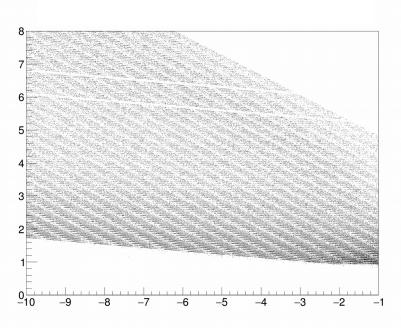
Strange striping observed in 3D hit distributions in new sensors
