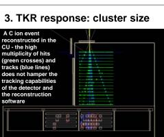
All the CU elements are shown in the reconstructed event: one TKR tower, 2 CAL modules and the top ACD tile are hit by ions while 4 ACD tiles and a complete TKR+CAL tower are not activated: the external container is also visible
