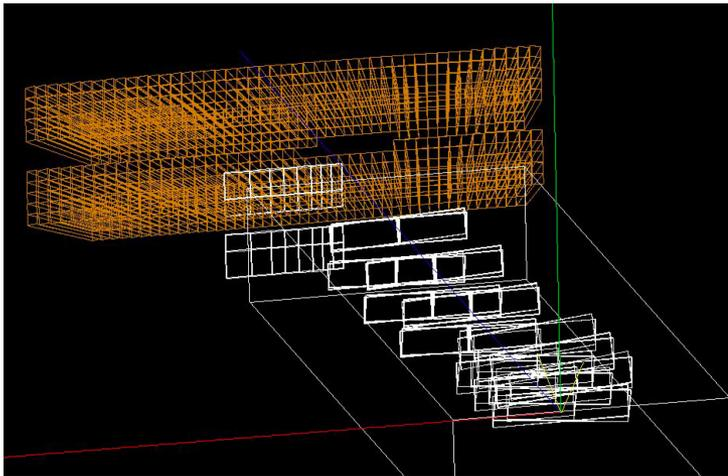
Scintillation hodoscope: double layer of scintillator strips for each half, with WLS fibers and maPMT readout
