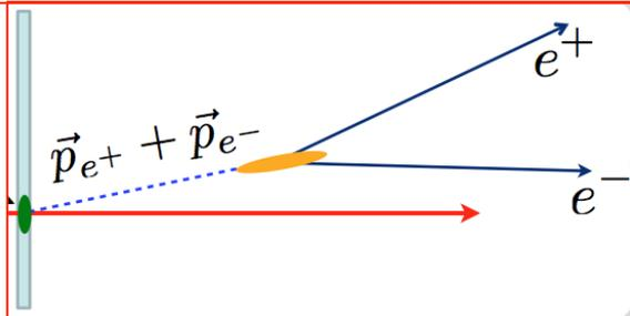
If  $\alpha'$  is small  $A'$  lifetime is long, many will decay downstream of the production vertex
