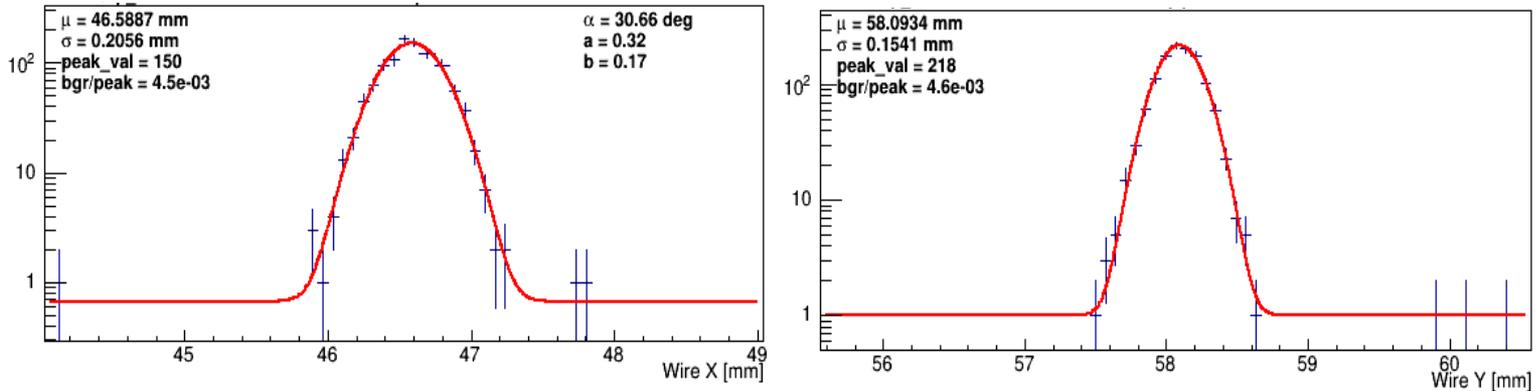
Beam position stability at 2H00 BPM with  $I_B \approx 50$  nA (Feb. 2-28)
