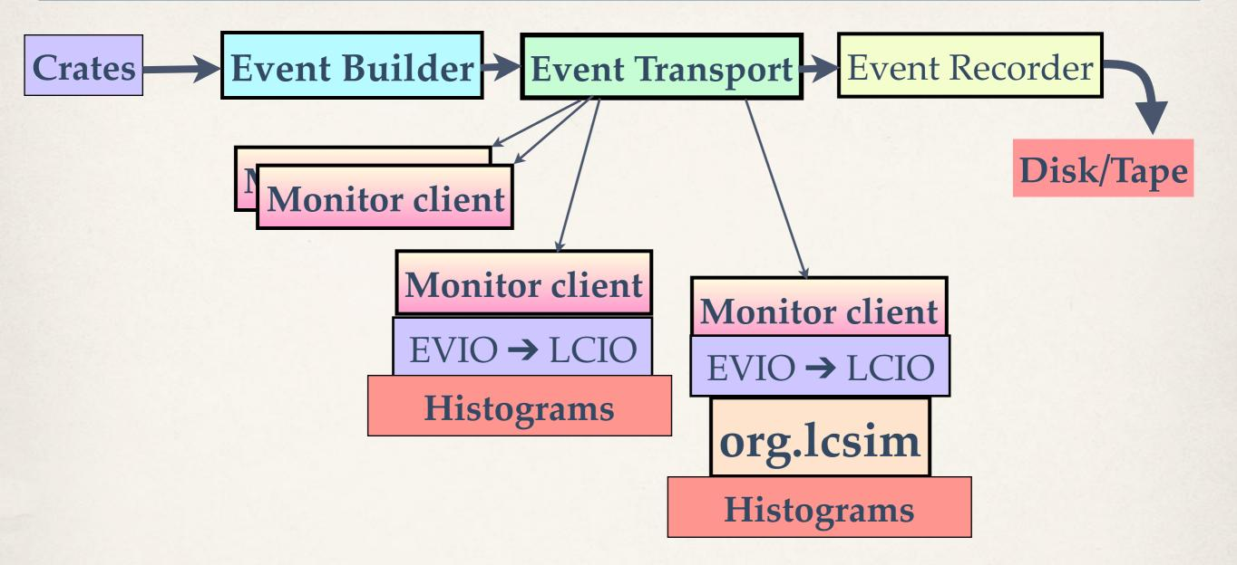
DAQ uses the EVIO format internally and for data storage of raw data. Event transport distributes and transports events.
