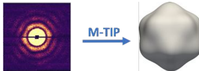
12nm reconstruction of an RDV virus from experimental LCLS data under icosahedral symmetry constraints
