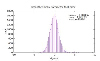
The Runge-Kutta extrapolation of the covariance matrix to the origin is not working perfectly, as the errors appear to be underestimated by several percent (despite being perfect at the first measuring plane).
