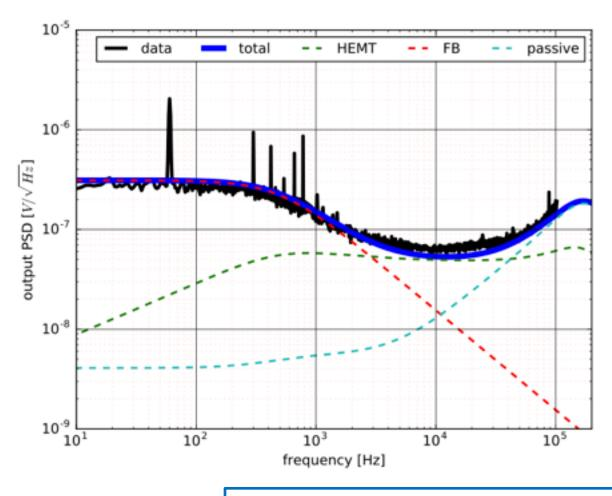
Charge amplifier noise at output
