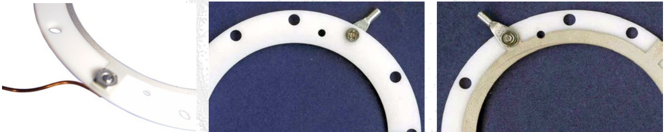
Figure 1.7: Connections to a ceramic ring. Left: cable clamped to a “front” ring (MCP side visible). Middle/right: cable clamped to a back ring with 3mm lug, countersunk M2 screw and special M2 nut.
