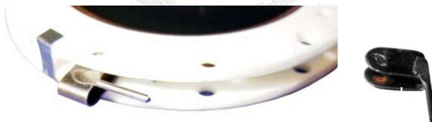
Figure 1.17: MCP stack with spring clamp for the MCP back cable (DLD40, DLD80 & HEX80)
