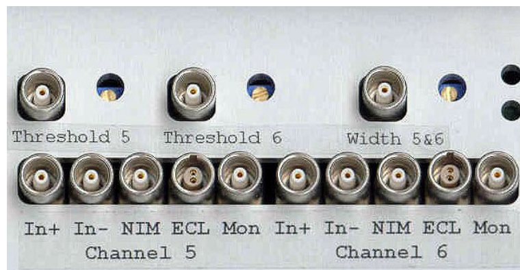
Figure 3.7: inputs, outputs and controls of the ATR19 for each internal DLATR board
