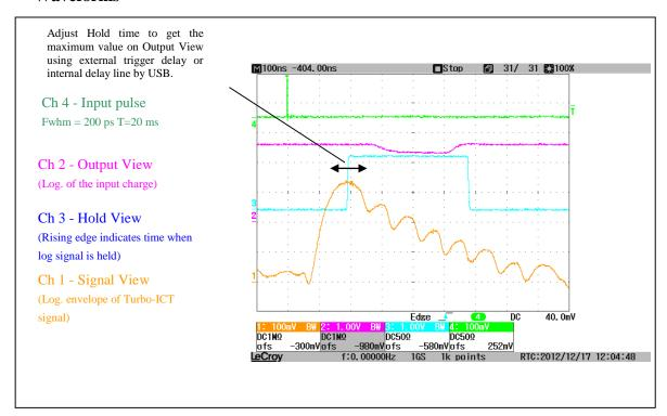
Channel 4 (green) shows the input short pulse which goes thru the Turbo-ICT aperture.
