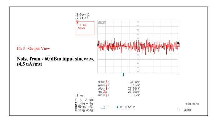
The noise (standard deviation) from -60 dBm signal applied through ICT-Turbo1 aperture is about 21 mVrms. The equivalent input noise taken from the calibrated reverse function is 0.14 uArms i.e. 0.7% resolution. Notice that the resolution remains the same although the signal decreases.
