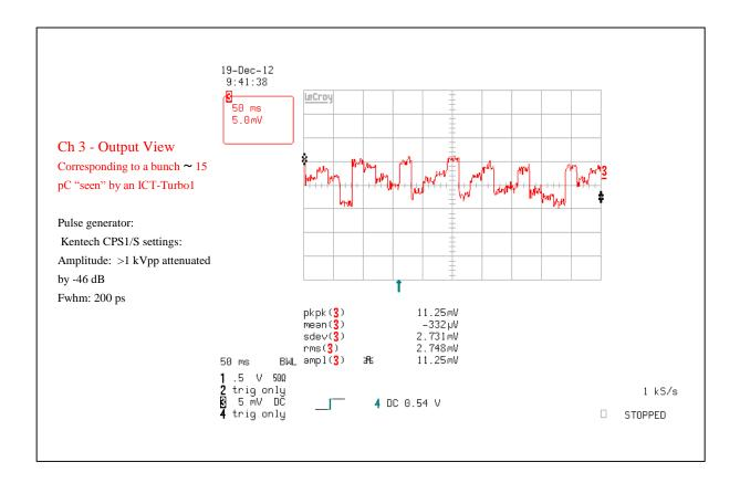
From a succession of 15 pC input pulses, the BCM-RF provides an output noise standard deviation of 2.5 mVrms. Applying the calibrated reverse "log" function from an ICT-Turbo1 to this output noise gives an equivalent input noise of 0.11 pCrms. One can see that the signal over noise ratio is 136, equivalent to 0.7 % resolution.
