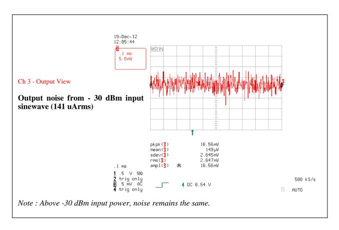
Output View contains ~2.7 mVrms of noise when -30 dBm signal is applied through the ICT-Turbo1 aperture.
