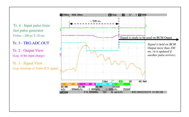
BCM Output signal is ready to be used on the rising edge of TRG.ADC.OUT which occurs about 500 ns after the input pulse.
