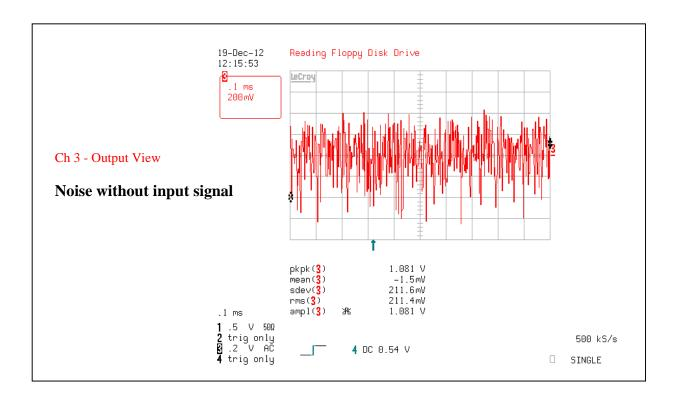
Without input signal, Output View is noisy because in the absence of an input signal the logarithmic amplifier gain increases.
