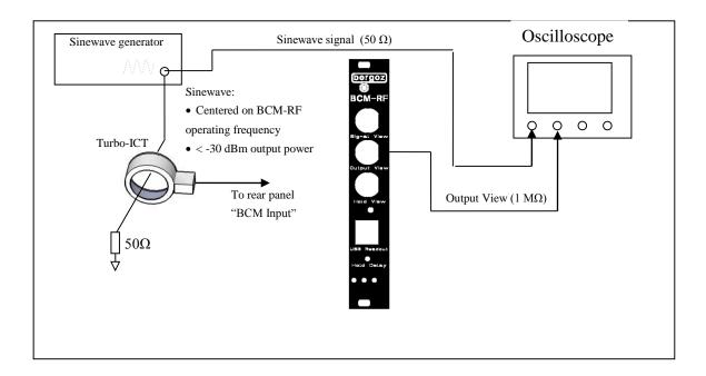
Connect the Turbo-ICT to "BCM Input" SMA connector on chassis rear panel.
