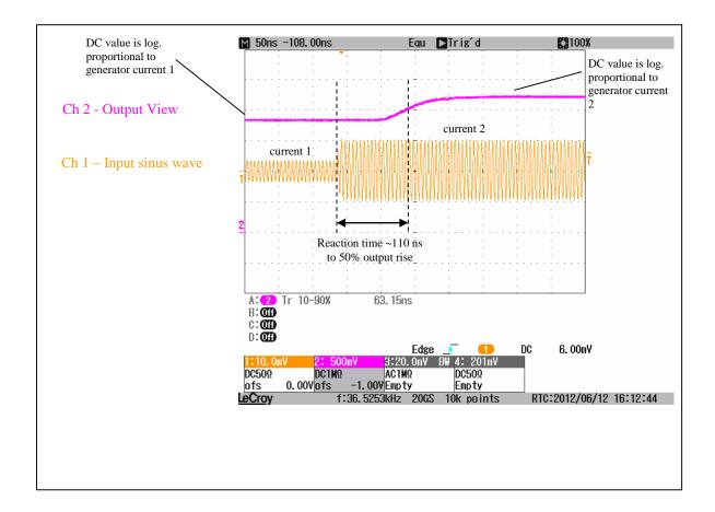
The signal Output View is proportional to the logarithm of the current from the generator.
