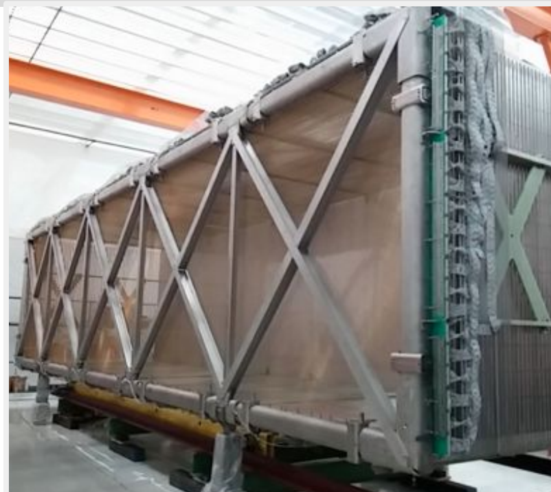
“Eyes” of the MicroBooNE detector -- a time-projection chamber,-- before installation
