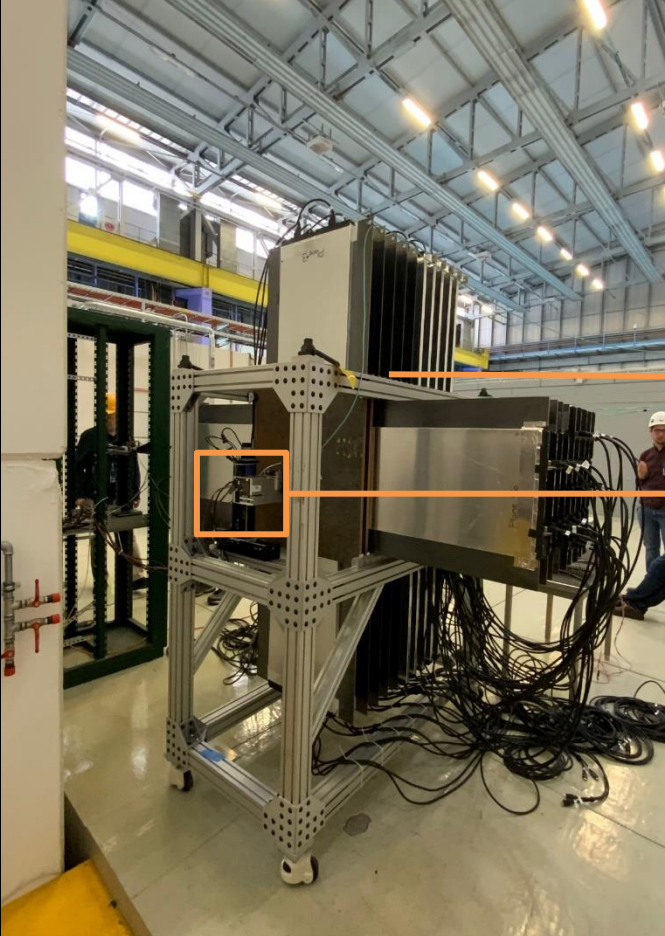
Hadronic calorimeter prototype with 19 layers of 25mm absorber and trigger scintillator prototype with two layers of plastic scintillator
