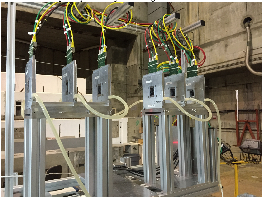
6 Mimso26 sensor planes plus cabling and cooling
