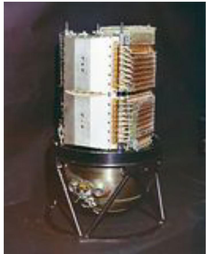
6 inch spark chamber
