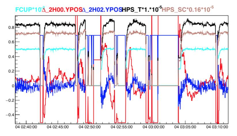
Very difficult to tell if this is actual beam motion, or the BPMs being inaccurate due to the trips.
