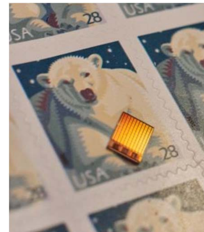
ePixS: a 100 channels signal processor for spectroscopy with a floor noise of 8 e - rms
