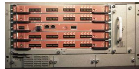
5-slot ATCA Shelf, but can have crate up to 14 slots
