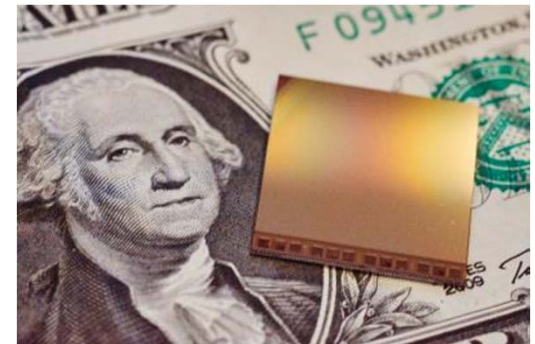
ePix100: 28 Million transistors. Bigger than an AMD Athlon K6 and slightly smaller than a Pentium 4
