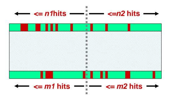
Only the first m1,2 or n1,2 hits are kept, where  $m, n \le 64$ The limit is adjustable by plane and end
