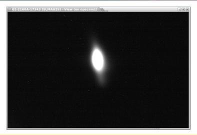
Beam image produced by the synchrotron light emitted in ArcA,  $E_{beam} = 9.5$  GeV, tune-mode beam.
