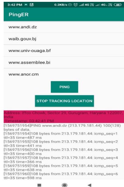
Fig 4. Ping output displayed in the application
